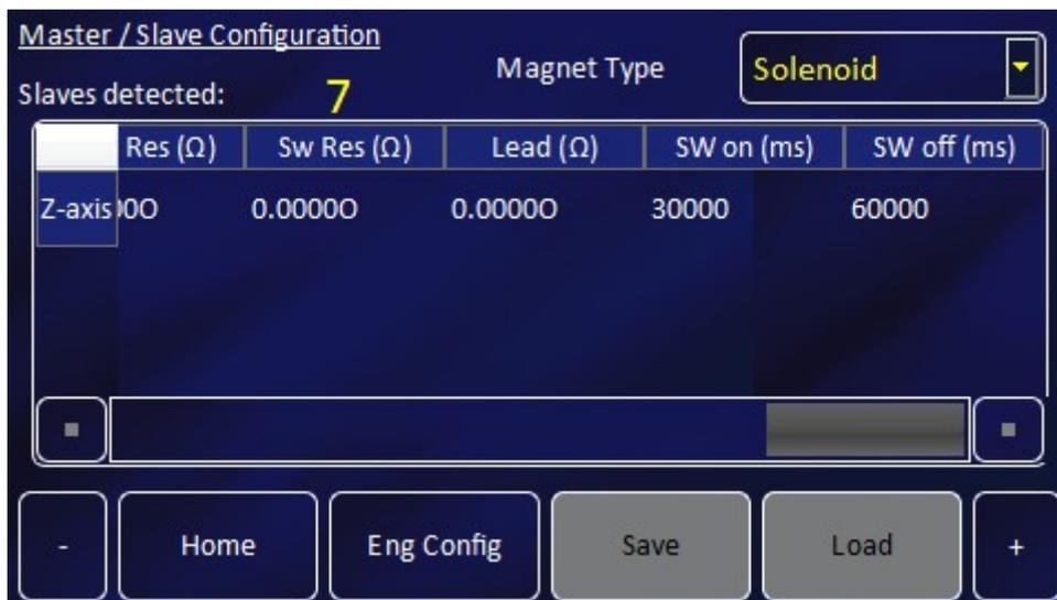
**Figure 1** Switch heater times configuration
